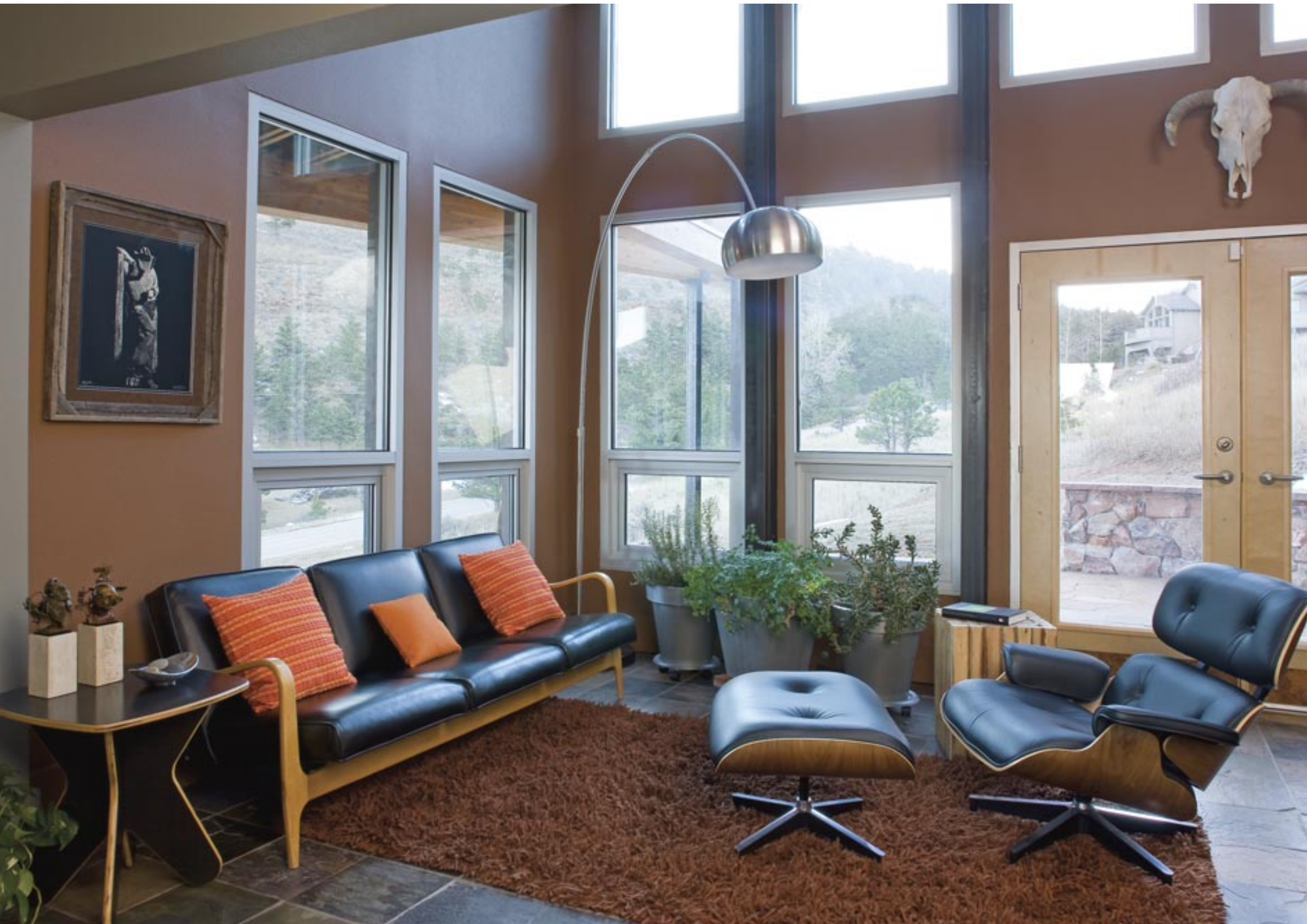
Sliding doors once separated the sunroom from the main house, but today, the room is a natural extension of the home. Ritter made the most of the room's double-height space, allowing sunshine to pour through the windows. Notice the steel columns, which reinforce the two-story wall while serving as a strong design element.
